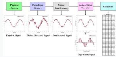
Digital Data Acquisition System Block Diagram
